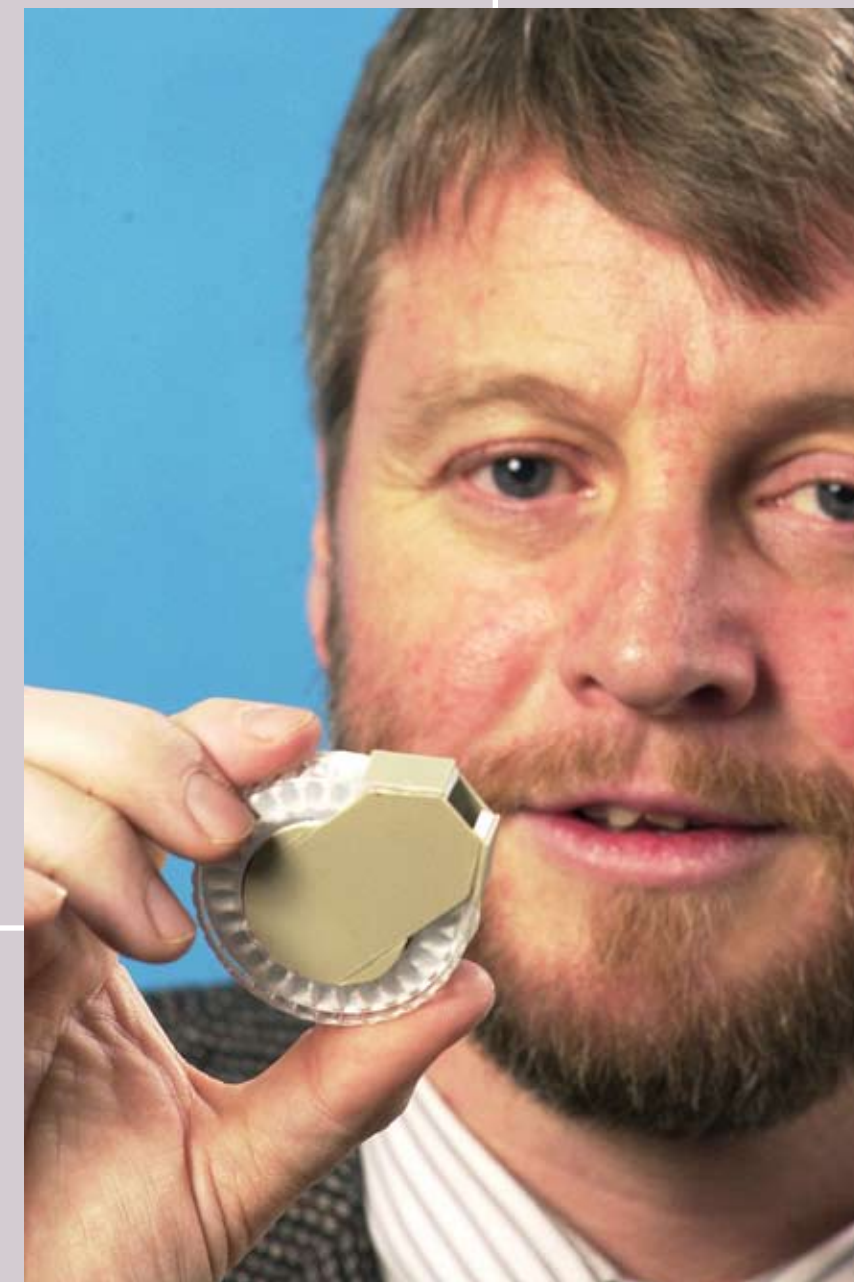
Unlike conventional inhalers, which deliver a constant stream of a drug, the Oriel device monitors the patient's breathing and adjusts the delivery of the drug to improve treatment.
