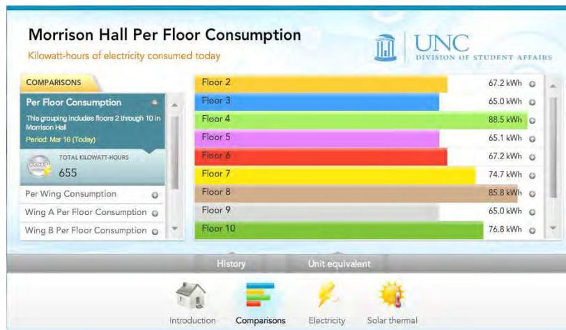
electrical energy use. The team commissioned the energy sub metering. Some of the HVAC meters were not able to read accurately as the energy use dropped, due to conservation efforts, below their design operating range. In response to HVAC metering problems, the dashboard was reconfigured to only display electrical energy to each zone. Building occupants have the greatest impact on electrical consumption.
