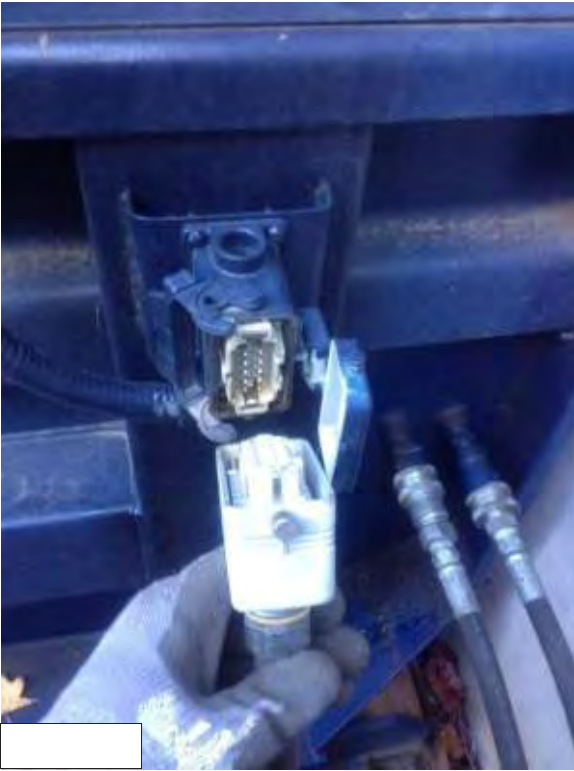
Electrical cord unplugged [Figure 8]
