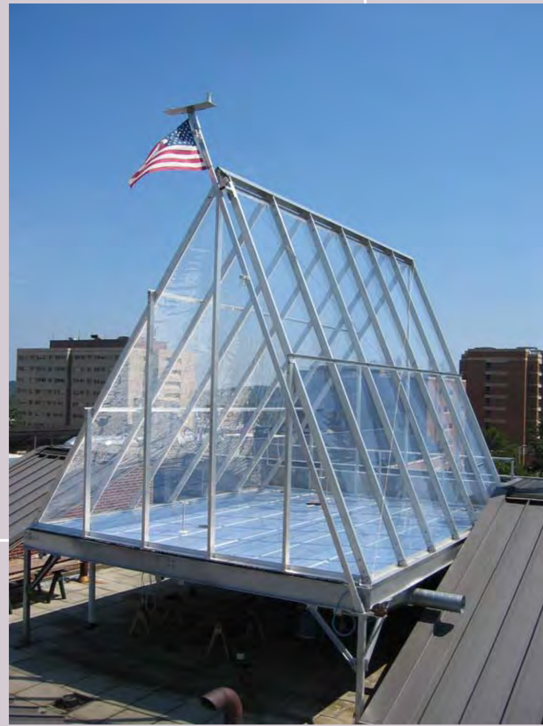
On the roof of the School of Public Health, scientists fill this chamber with synthetic smog and place lung cells inside it to investigate the effects of air pollution. The chamber is connected via a large tube to the research laboratory on the building's top floor.
