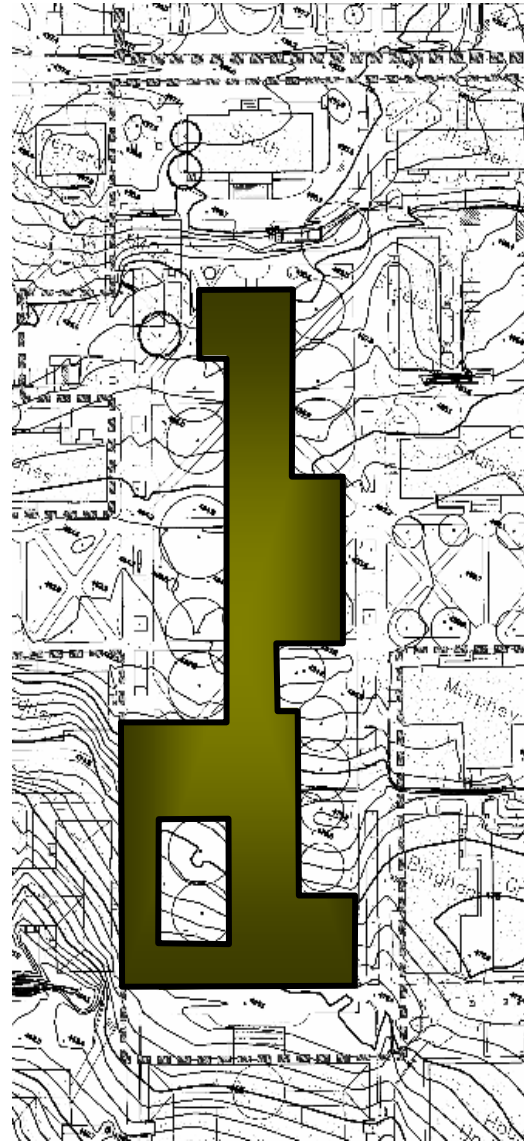
Area to consider creation of impact resistant lawn soil over Silva Cell tree
