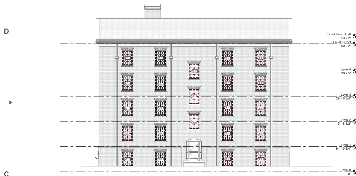
C1 PLAN WEST DEMOLITION ELEVATION 1/8" = 1'-0"
