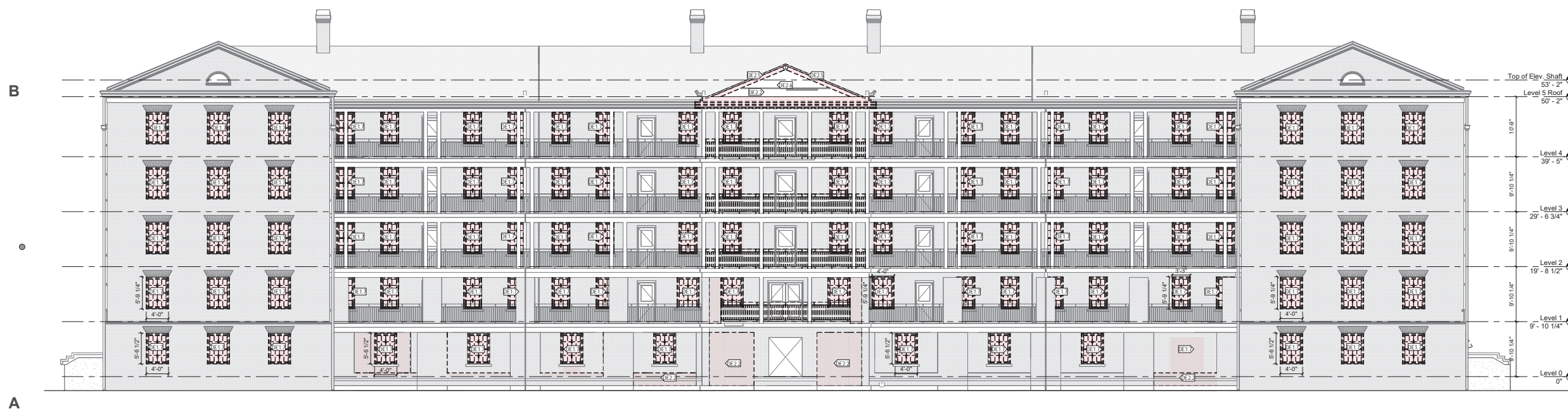
A1 PLAN SOUTH DEMOLITION ELEVATION 1/8" = 1'-0"
